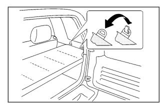
Use the anchors in the rear of the vehicle to hook the cargo cover in place.
